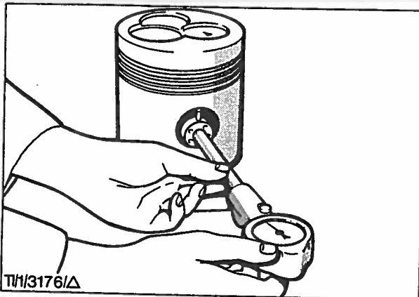
Fig. 34 - Measuring Piston Pin Bore
